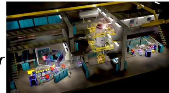
Two accelerators  $\rightarrow$  50-400kV [300-3MV] with high ion beam currents: 100 mA proton, 50 mA helium [ $\geq 1\text{mA}$ ]
