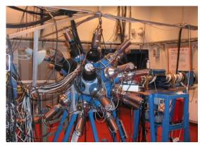
SiRi: 8x8 Si  $\Delta$ E-E particle detectors ( $\approx$ 9% of 4 $\pi$ )
